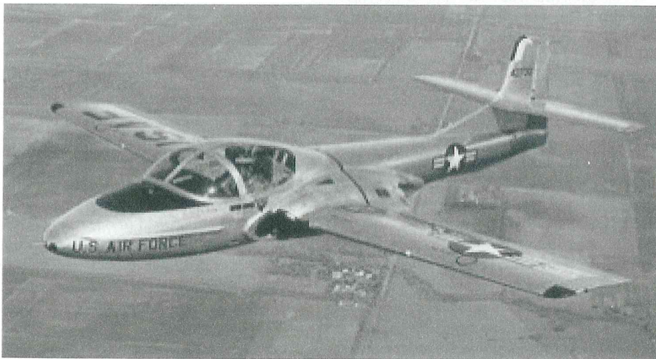
Opposite: the RAF's Percival Jet Provost which flew initially on 16 June 1954 employed side-by-side seating, later adopted for the Tutor. RAF. Top: the compact Tutor configuration is seen to advantage in this shot. CANADAIR. Above: the Cessna T-37 first flew in October 1954 and also seated instructor and student side-by-side. AUTHOR.
